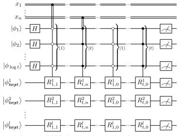
Figure 3. A Quantum OBDD for computing Boolean function given by its linear characteristic.
